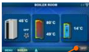
Boiler ON/OFF (position when boiler is switched off)
