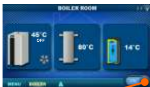
Boiler ON/OFF (position when boiler is on)
