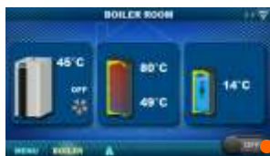
Boiler + Buffer tank + DHW
