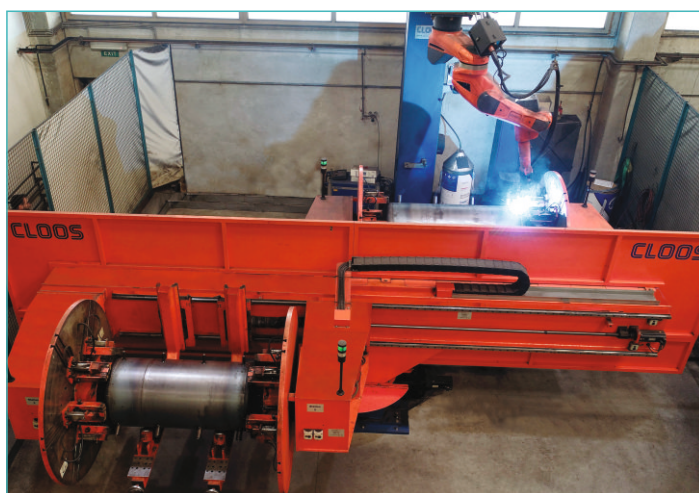
Robotic welding of stainless steel water heaters
