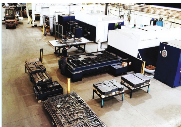
Cutting of metal sheets using modern laser technology
