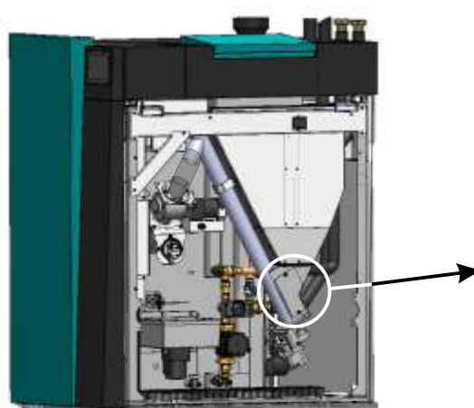
2. Unscrew 2 screws and open side cleaning lid of the pellet tank.
