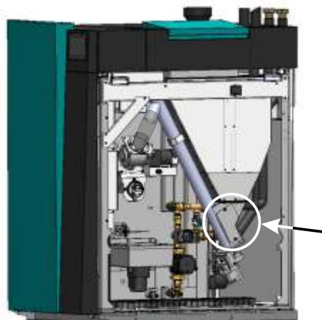
4. Close back cleaning lid of the pellet tank airtight with screws.
